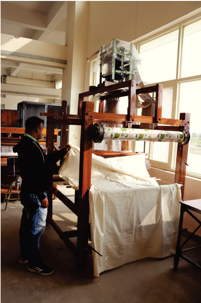
Routine maintenance of Jacquard Loom being carried out by Technical Instructor
